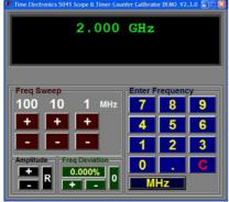
precision closed-loop output level control up to 2.2GHz suitable for calibration of high-frequency oscilloscopes or counters
